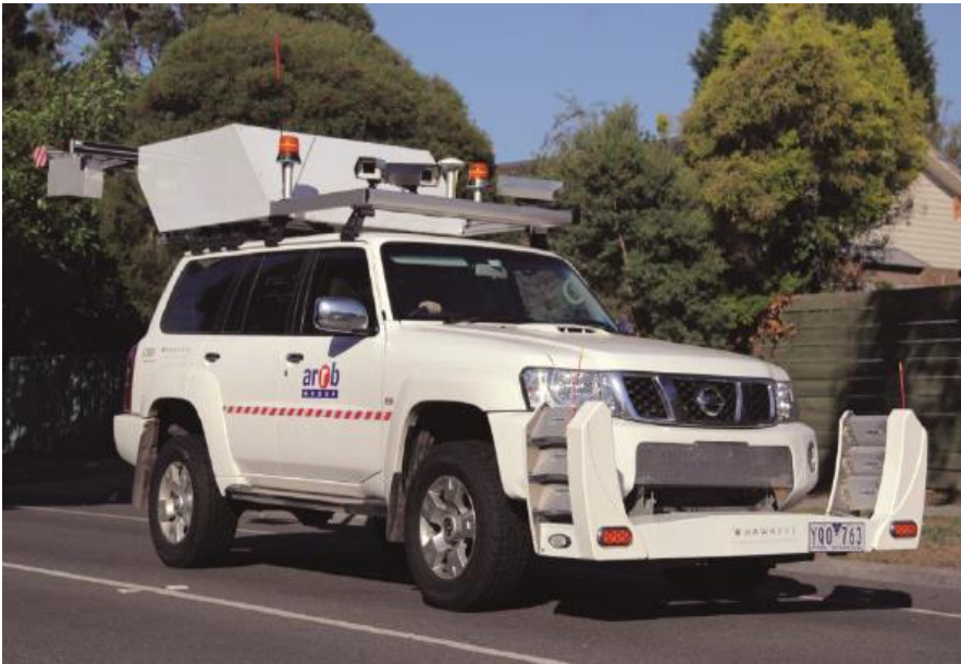
Figure 1.3: Network survey vehicle (NSV)
