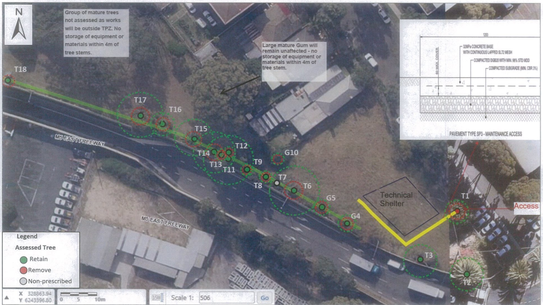
Figure 7 – Princes Highway interchange. Scaled aerial mapping marked up by [red dotted circles] Red dotted circles denote SRZ, TPZ noted with green hashed circle.
