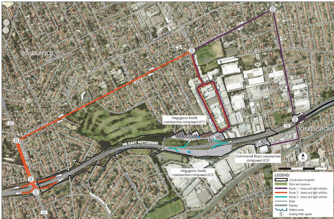
Figure 1: Approved heavy vehicles routes for the Kingsgrove construction compounds (from SPIR, Figure 6-2)
