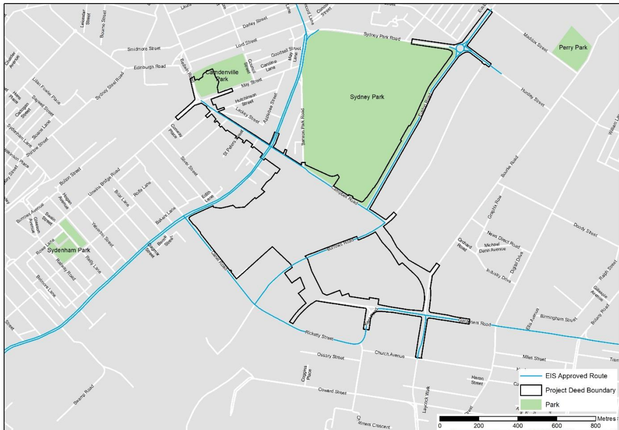
Figure 1: Heavy vehicles routes identified in the EIS for access to the St Peters Interchange and Local Roads Works construction areas
