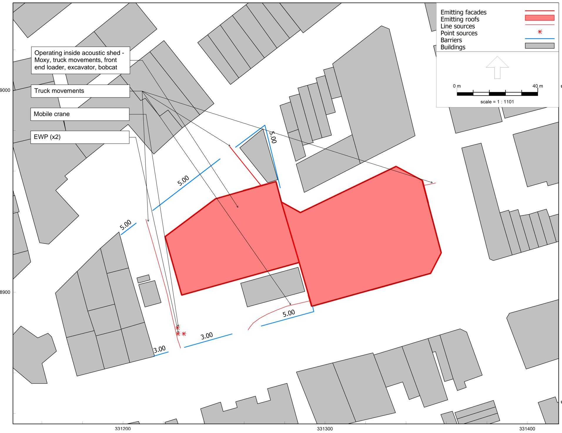
**Figure B.1****Modelled equipment locations – Stage 1**
